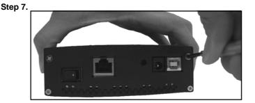
Replace the two screws which were removed in Step 1 from the back of the VPA-3528Net NetWork Storage.
